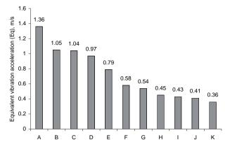
**Figure 2.** Equivalent frequency corrected vibration acceleration values for various field and transport work activities (mean values; direction – Z) registered at: A – tedding and raking of hay; B – grass mowing; C – fertilizer spreading; D – soil aggregation; E – cultivation; F – cutting carrot tops; G – potato digging; H – sugar beet digging; I – cutting and grinding maize; J – sowing grain; K – driving along a field road.
