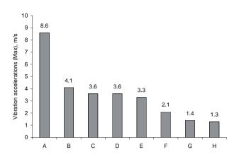
Figure 1. Maximum acceleration values on tractor seats according to the type of work activities (Z – direction) registered at: A – fertilizers spreading; B – aggregation and discing of soil; C – transport and manure spreading; D – tedding and raking of hay; E – cultivation; F – potato digging; G – sugar beet digging; H – driving along a field road.
